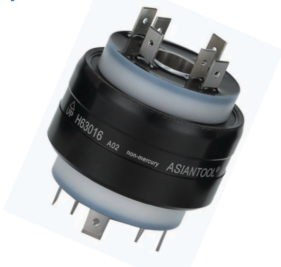
H63016 NM (non-mercury) 6poles/30A/AC250V Through-bore:16.2mm
