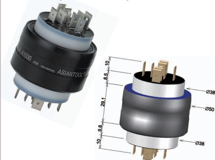
A1030 8poles/30A& 2poles/4A AC250V
